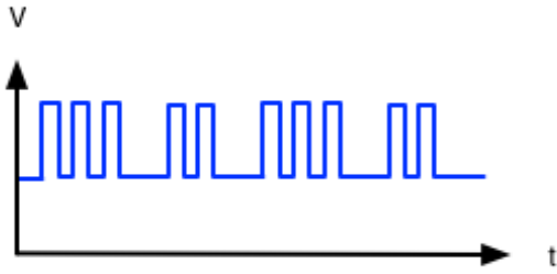
Figure 1: The tag modulates the magnetic field at a frequency of 13.56MHz, transmitting data to the reader. In this figure, a conceptual representation of this effect can be seen. The high portions represent transmission of a '1' while the low portions represent transmission of a '0'.
